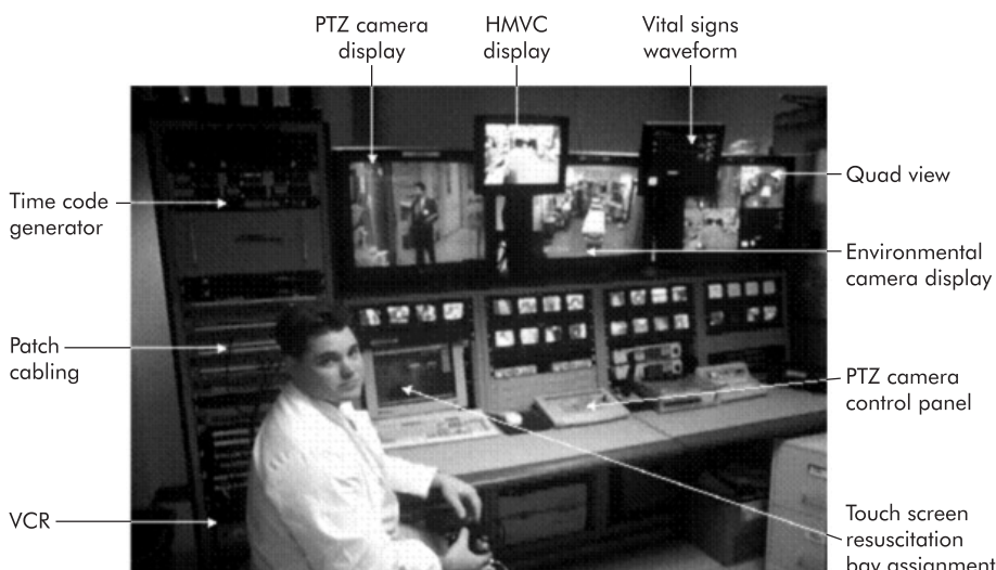
Figure 2 Telecontrol centre showing three full screen displays above 28 small screen individual camera images. The right full screen displays the "quad" image. The two stand out screens between the full screen monitors display the vital sign waveform data (on right) and the wireless head camera image (on left). The touch screen panel (above keyboard) allows the video technician to display any one of the video instrumented locations with a single key touch. The time code generator and patch board is shown to the left of the video technician. Four video cassette recording machines (VCR) are arranged in the rack beneath the video patch board.
