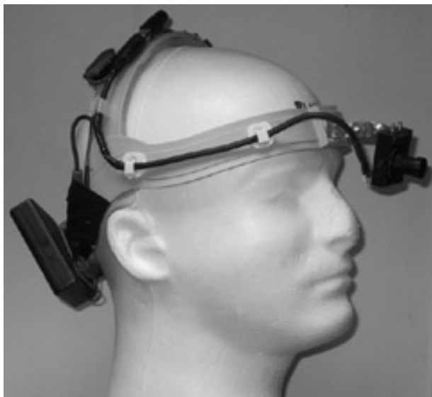
Figure 4 The wireless head camera had four AA batteries in a box mounted over the occiput. The camera was on a swivel mount between the eyes. The video transmitter was positioned in the middle of the 10 resuscitation bay trauma resuscitation unit layout and allowed free range movement with image transmission over about 100 feet.
